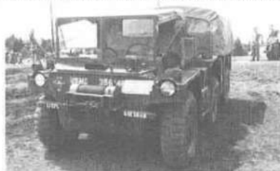
■ M561 At the time of the picture, this M561 Gama Goat was part of the 3rd Marine Division. Note the position of the winch on the front of the vehicle.
