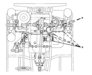
GAA Upper and Lower Suspension Ball Joints (2 fittings) (See note 13) (LV-Q) (O)
