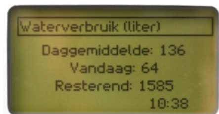
Afb. 10.1.6 – 4 Display van een microprocessorgestuurde ontharder -> Display of a microprocessor controlled water softener, reading (top to bottom): average daily waterconsumption, to-day's consumption up to now, remaining volume till regeneration (all in litres)
