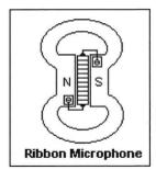
Most significantly, we now have a sensitivity that is proportional to  $\cos \theta$ . The ribbon microphone is equally sensitive to sound coming from front and back (so two people can face one another across it and both be equally heard), and is completely insensitive to sound coming from 90° or 270°. This pattern is not dependent on frequency, as are diffraction effects. The ribbon microphone discriminates by a factor of 3
