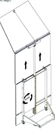
6. Push the Upper Panel against the magnets. Turn the Crank in the opposite direction to lower the Upper Panel until it rests on the Lower Panel in the Performance Position.
