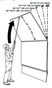
5. Turn the Crank clockwise to raise the panels. The Crank will stop when the panels reach the tower's maximum height.
