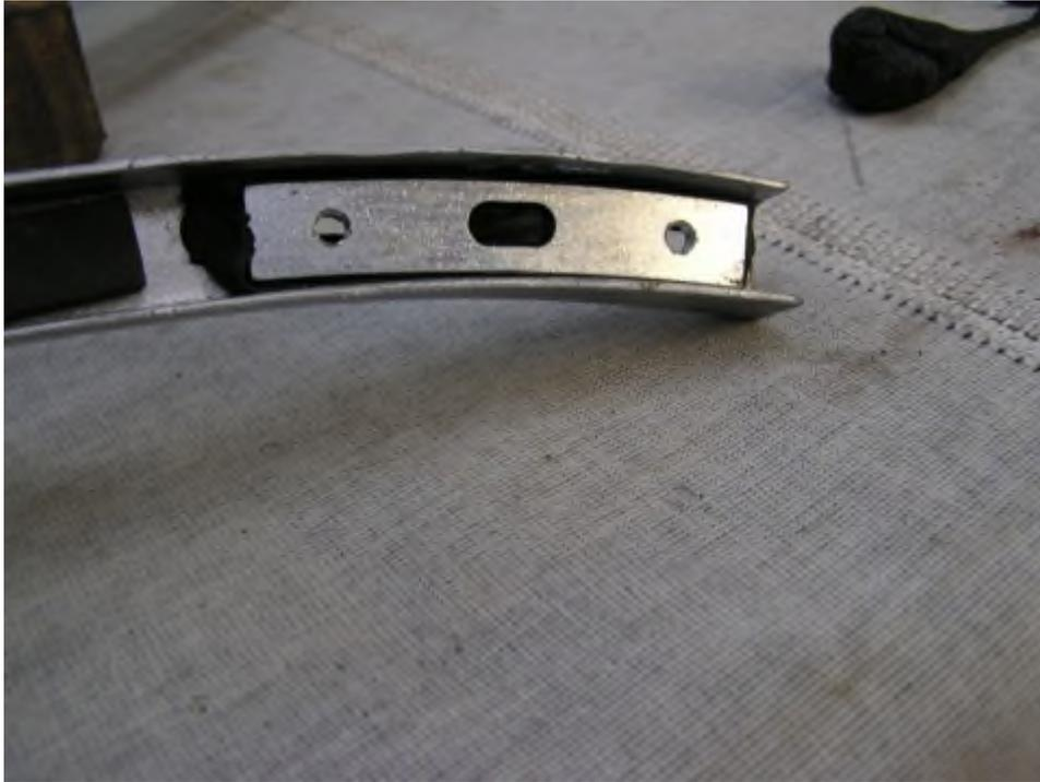
Also check the holes for the header trim mount screws. If enlarged, use pliers to squeeze the holes tighter. It's just soft steel and usually re-forms itself.
