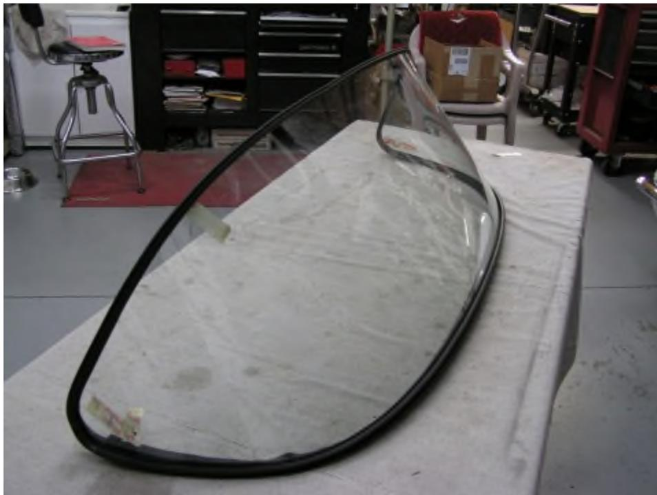
When installed, take your rulers to ensure the inner rubber flaps are in proper position. This is important to get them to fit over the inner chrome post flanges at the dash pad on both sides. I use 2 rulers, one on edge against the vertical glass edge, the other ruler to measure the edge of the flap. Get them both equal by moving the rubber as needed.
