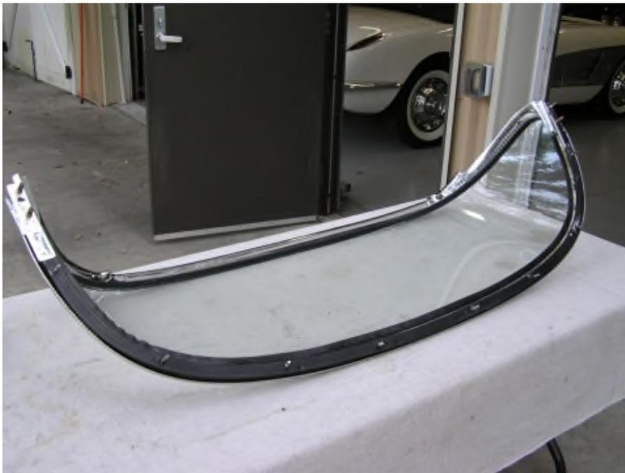
If you are replacing the glass, skip this step. If you are re-using the glass and just replacing hardware or the rubber seal, use masking tape on the glass at various frame channel and side post endpoints and mark them in ink for later reassembly. Mark the endpoints of the frame channels, post inner flange tabs, and other various points. It's also recommended to place some marks on the glass and upper/lower channels for alignment.
