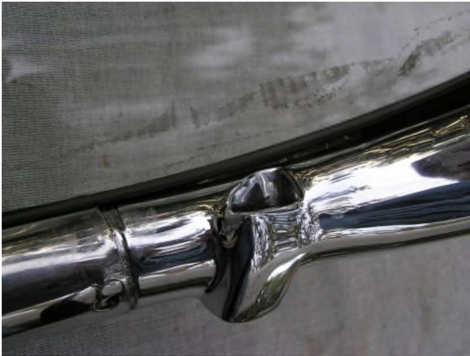
Once you get the post a bit free from the upper channel, carefully pull the end out and away from the rounded header trim. This metal to metal attach point may have some corrosion and rust so you may need penetrant to help free it up. This frame wasn't bad so it came out relatively easy.
