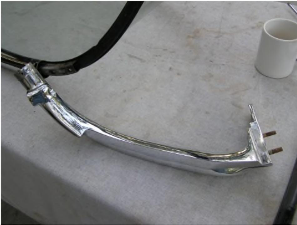
Now begin to remove the lower frame channel trim assembly from the glass rubber seal. Carefully pry the ends away and remove the assembly from the glass. Keep track of the 8 T-bolts and remove them for later cleanup and reassembly. There will be 2 nut plates held into the channel ends with clay sealer.
