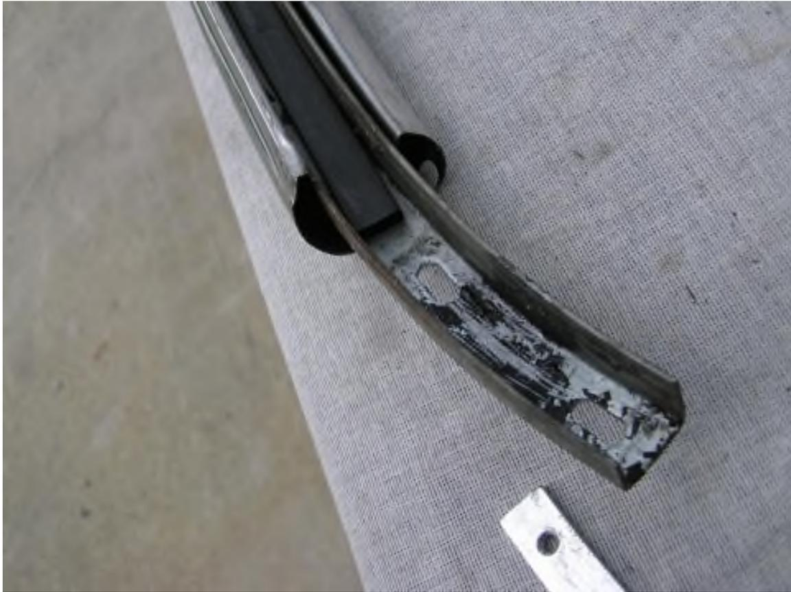
Here you can see how the header stainless trim is captured by the frame channel. This must be separated later for reassembly. The lower trim lip can be seen clipped over the channel edge. Tricky to remove, but doable with a procedure I use. More later on that.
