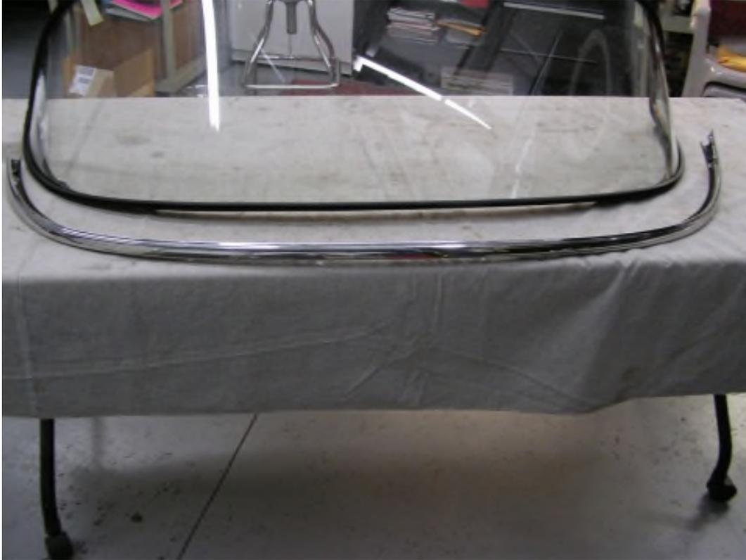
Here you can see the narrow nut plates for attachment to the side post tabs. Use dum-dum clay sealer to hold them in place on each end of the frame channel.
