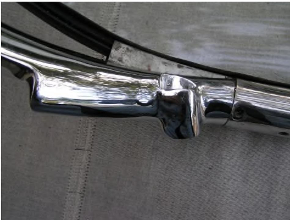
Do the other side next. Here you can see the channel ends exposed and the mating area of the post. Keep in mind, if you send your posts out for re-chroming, make sure they are aware that they must NOT leave slag and extra plating in the channel slot of the post. Too much copper and plating build up in this area will cause much difficulty on reassembly. The same area to be protected from extra plating material is the side area where the lower stainless trim meets.
