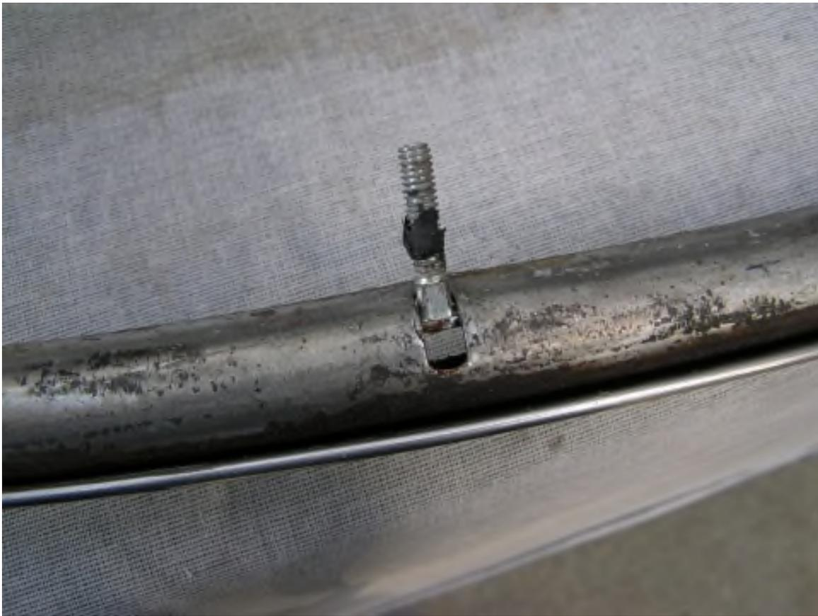
Remove the upper header frame channel from the glass. There will be a nut plate at each end of the channel, used for those 2 integrated washer screws above, normally held in place with a clay-like non hardening sealer(dum-dum).
