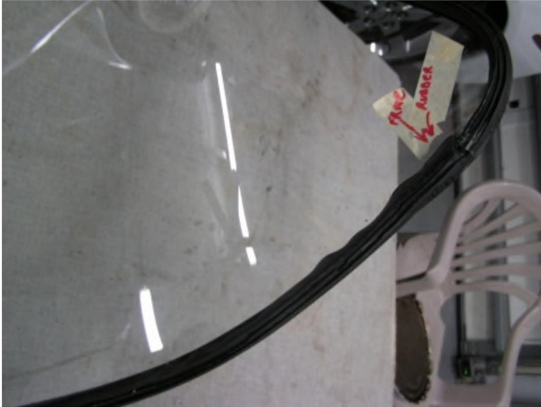
Now that all of the hardware is removed, you can peel away the rubber from the glass. There may be old hard sealer there from original installation or a replacement shop. Clean everything up for reassembly later.
