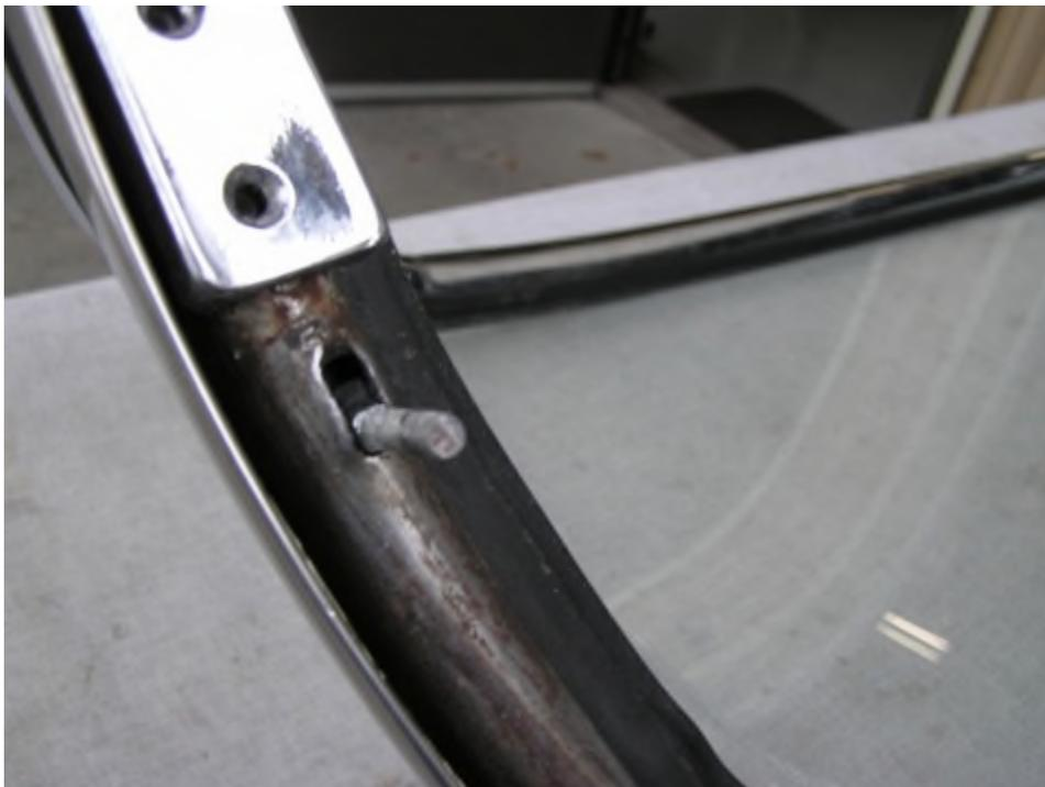
Continue to remove the other side post hardware. Keep track of all hardware for reassembly.
