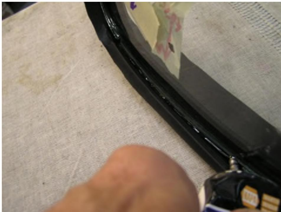
Lay the glass on the table with the top edge down, and using your soapy water solution, liberally brush it on the entire lower surface of the rubber seal, particularly along the ribbed edges of the seal. Don't be shy with the amount. Soak it up good as it'll dry up a bit as you install the channel. I avoid oily products here as they wont dry and damage the rubber over time.
