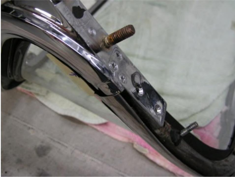
Line up then loosely attach the 2 screws holding the post tab to the lower channel. Note: DO NOT use sharp objects to line up the nut plates and tab or upper post holes. Use a blunt tool with a dull point. If you use a sharp tool it may hit the edge of the glass and break it.
