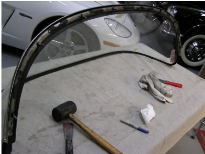
When everything checks out, get some wooden blocks and rest the assembly bottom edge down, carefully keeping pressure away from the T-bolts. I use 5 blocks.
