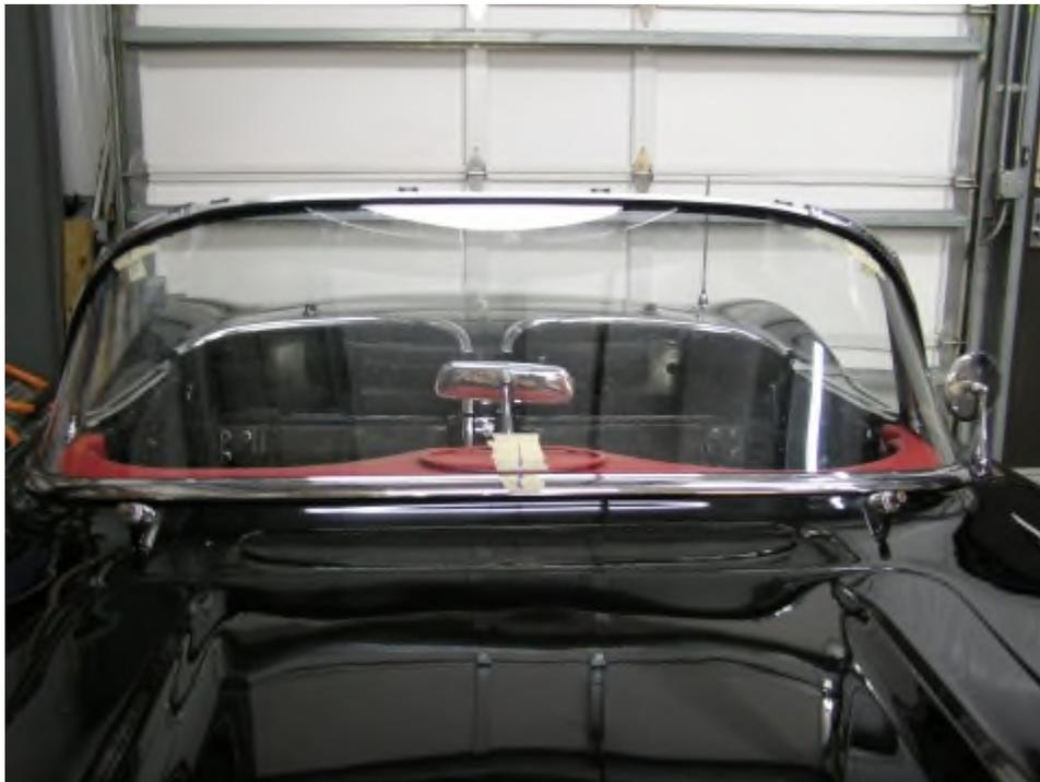
Notice the wrinkle free inner corners and the equal alignment of the end flaps over the inner post chrome flanges. All of the prep work and planning helps make a very time consuming project a "one-time" treat when it's completed!
