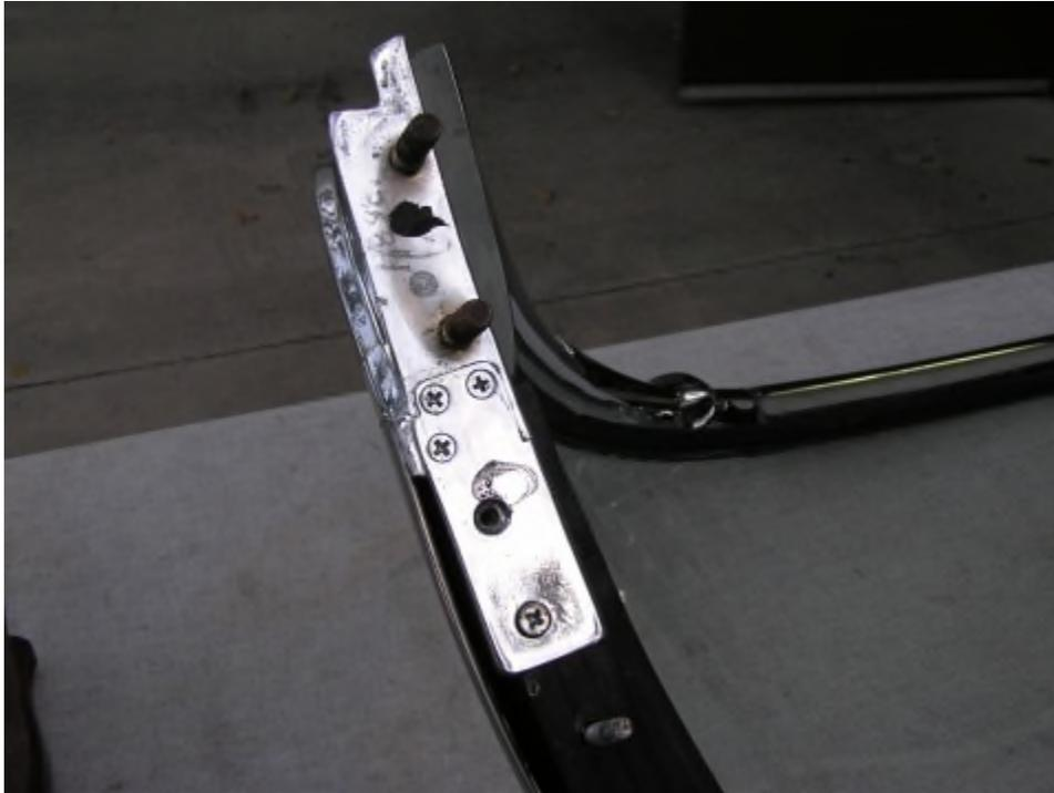
Both frame attach screws removed, and the trouble T-bolt you got at under the dash can be seen.
