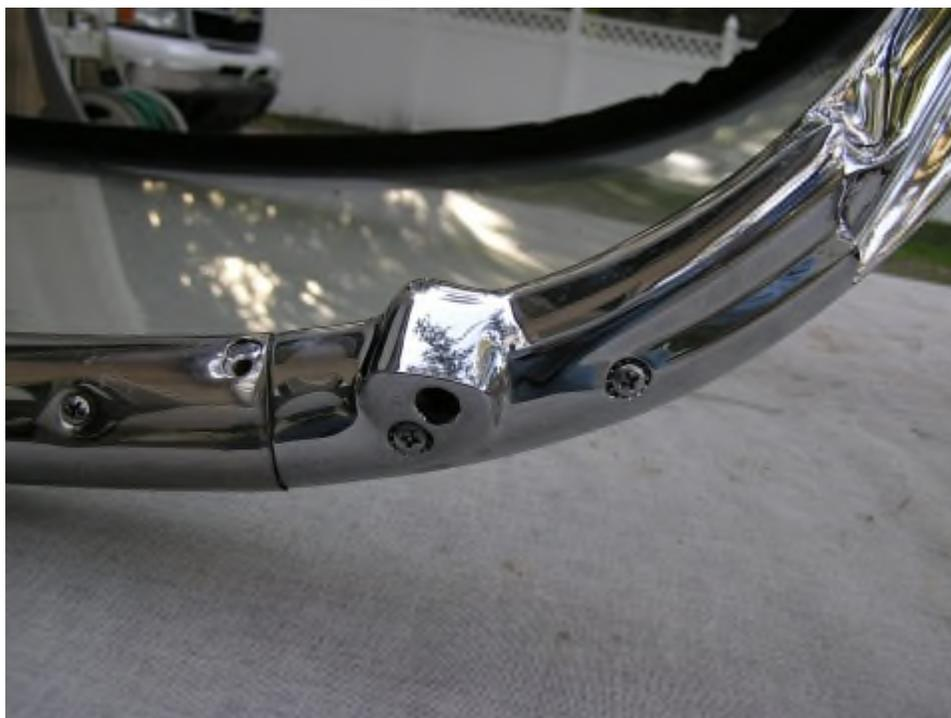
Also remove the 4 small screws securing the header trim to the header frame. One is shown on the left.
