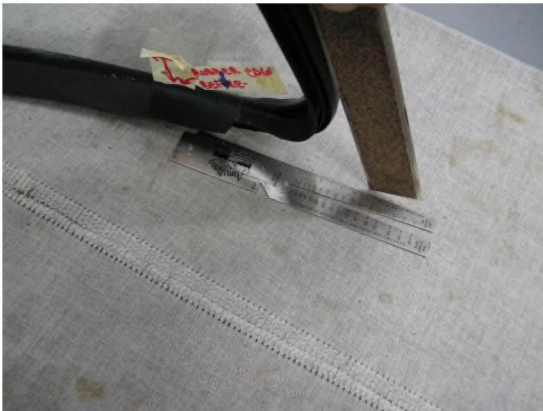
Now mark the center of the glass if you haven't done that earlier. I used the string method on this one, starting and ending at the edges of the rubber flaps which were evenly spaced. Find string center by folding half way, then replace on the glass and mark the glass center. Also mark center of the lower frame channel and it's trim by using the tape measure to find center.
