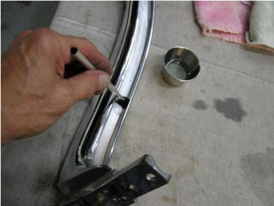
Note here that the side of post will be fitting under the lower trim. Carefully get into position as you install the post. It will later snap over the lower lip of the post.
