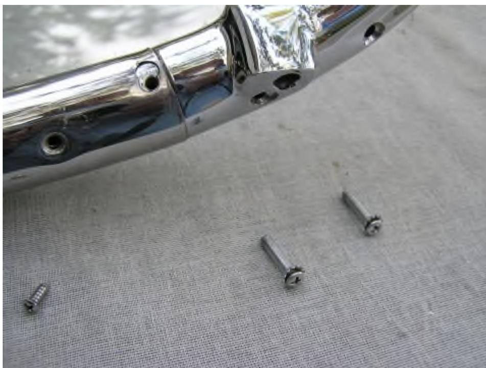
Using a pry tool, carefully begin to separate the post from the lower channel. Pry it just enough to get the post moving from the rubber. Then move to the upper frame and carefully pry the post from that.
