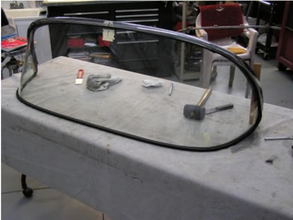
Now take some measurements of the edges of the lower channel to the flat table. Use your ruler and measure up to each edge. It should be very close on both sides. If not, recheck your glass & frame center lines. This is important for proper final assembly to get the rubber flaps and posts lined up.
