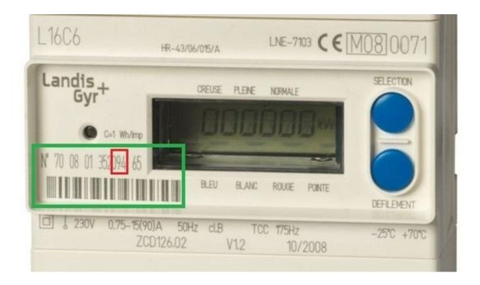
Meter readings, energy consumption, the lower blue push button called "defilement".
