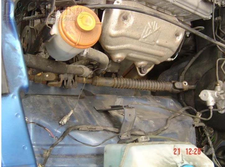
now drill out the bushes from the steering bar and install the 2x M80x80 mm bolts with bushes like shown on picture.
