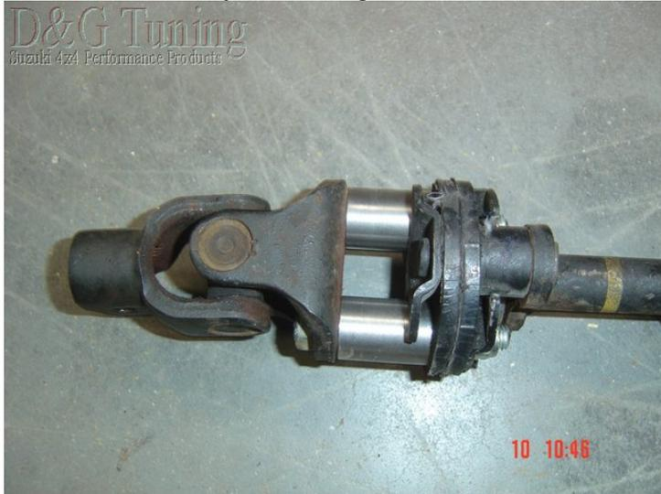
After you have installed the bodylift, install the steering bar again.
